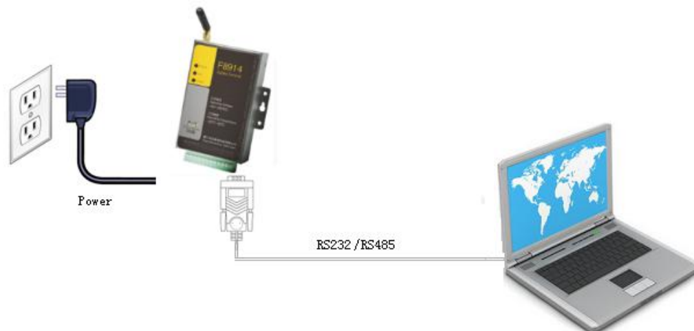
Figure 3-1 F8L10T configuration connection with PC
